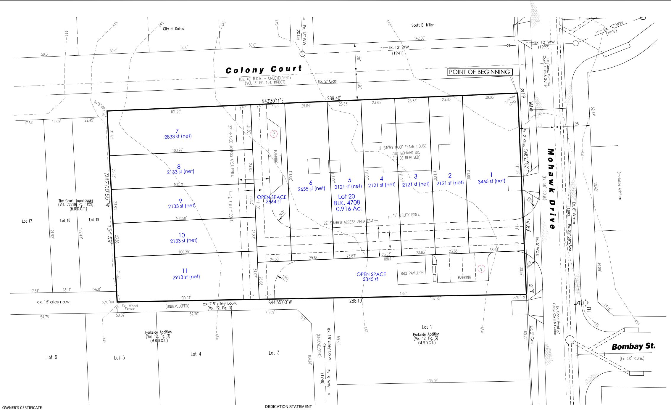
LEGEND 5/8" IRON ROD SET WITH YELLOW CAP STAMPED "RPLS 3963" IRF IRON ROD FOUND CM CONTROL MONUMENT 3 1/4"AD 3 1/4" ALUMINUM DISK STAMPED (SEMPCO SURVEYING) 60D 60D NAIL FOUND IN STEEL FENCE POST AC ALUMINUM CAP U.E. UTILITY EASEMENT D.E. DRAINAGE EASEMENT B.L. BUILDING LINE INST. NO. INSTRUMENT NUMBER DOC. NO. DOCUMENT NUMBER DRDCT DEED RECORDS, DALLAS COUNTY, MRDCT MAP RECORDS, DALLAS COUNTY, OPRDCT OFFICIAL PUBLIC RECORDS,
